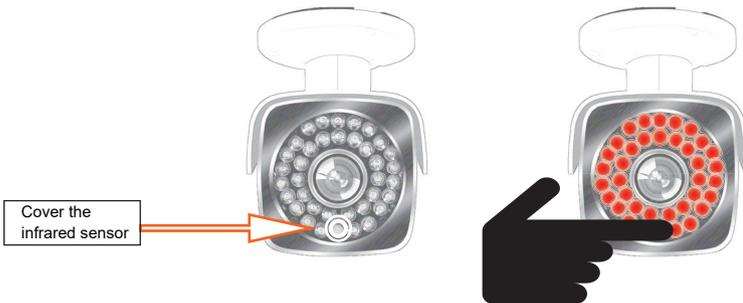
2)If the infrared lights don't turn to red in the dark,there may be a problem with the camera's power cable or power supply adapter.
